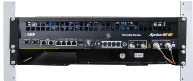
Rack mounted Aprisa SRi Protected Station with duplexer
